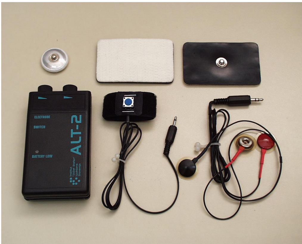
Figure 1: ALT-2 stimulator set with water-soaked electrodes, electrode cable and manual switch.
