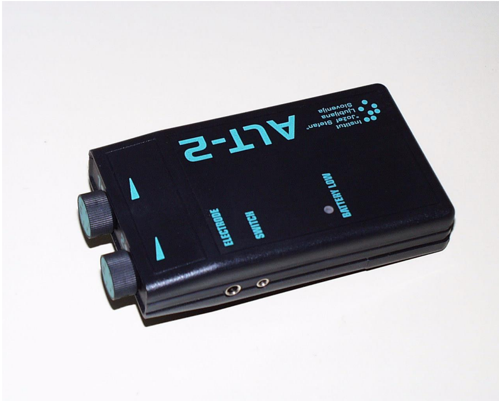
Figure 3: ALT-2 stimulator showing the position of stimulation intensity knobs and sockets for electrode connector (ELECTRODE) and manual control switch (SWITCH) connector.
