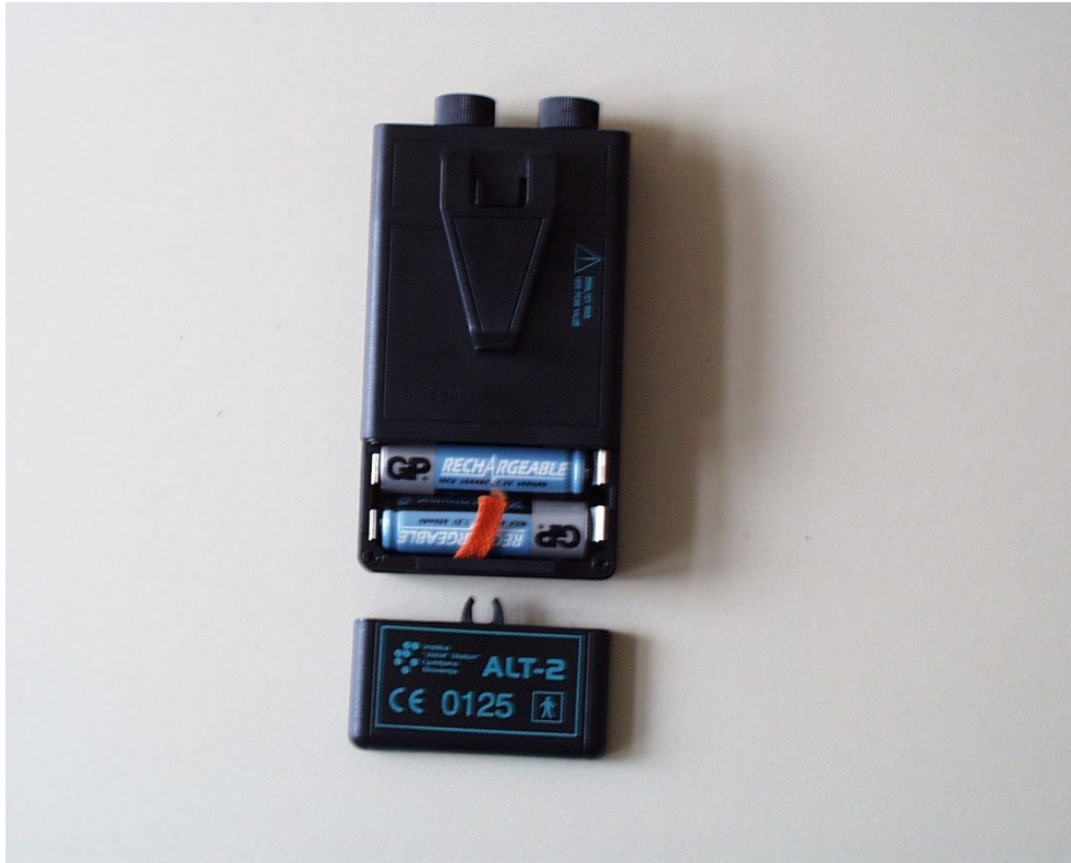
Figure 5: ALT-2 stimulator with open battery compartment showing the position of batteries.
